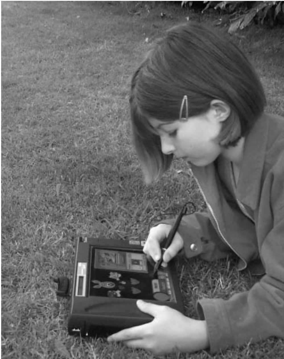
Figure 6. The concept HandLeR running on a Fujitsu Stylistic tablet computer with a Nokia GSM card phone
